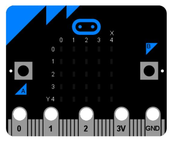
Some of the pins are bigger than others so it's possible to attach crocodile clips to them. These are the ones labelled 0, 1, 2, 3V and GND (computers always start counting from zero). If you attach an edge connector board to the device it's possible to plug in wires connected to the other (smaller) pins.
