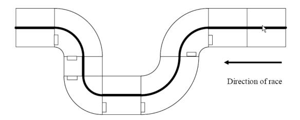
Fig. 4 Corner Markers Indicating Change of Curvature
