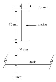
Fig. 5 Marker Position and Dimension
