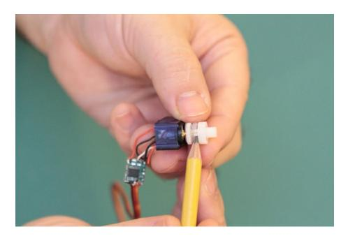
Gently pull out the gears and potentiometer. Minimizing movement of the press-fit gears now will mean a more solid / reliable gear-motor later.
