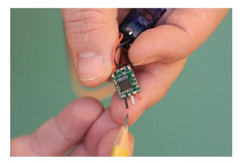
Touch the wires with a hot soldering iron and brush them away.
