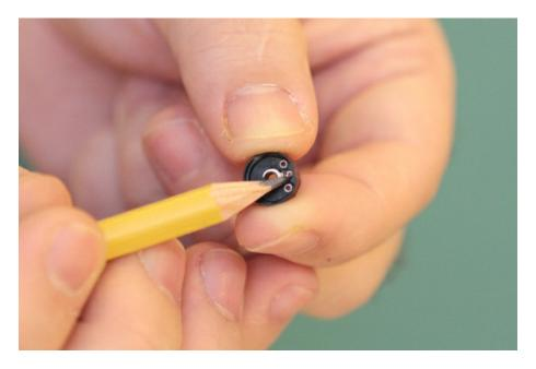
This... is a better way to fly. The foil contact and limiter are pressed into place - give them a little wiggle towards the gears and they should come right off.
