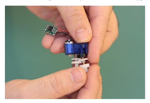
Push the potentiometer back into place carefully. Don't try to rotate the gears at this point, it's highly likely that you will damage them if you do.
