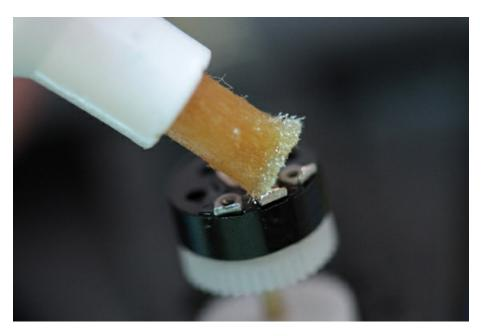
The potentiometer housing is typically heat resistant, but don't linger there too long. Just make sure that a little solder gets down to the rivet and call it good.
