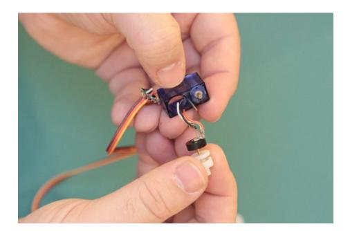
Clip them as close as you can to the base of the potentiometer. Try not to damage the housing, it's typically made of brittle resin or plastic.
