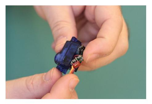
Make sure that the servo wires aren't pinched... and then re-insert the screws.
