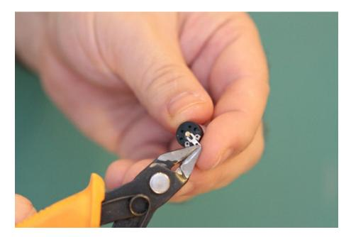
These bits on the shaft makes the potentiometer work... some of it will have to go.
