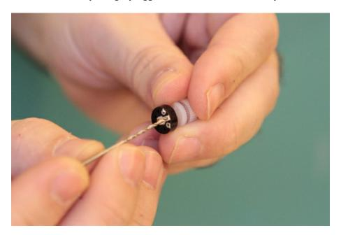
You can drill fast... but don't press hard. Also, try not to get any of the gear grease on this contact.
