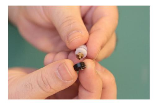
These little bumps in the potentiometer housing also help prevent continuous rotation. Many of the other hacks I've seen just have you break a chunk off... and re-assemble the servo. Compromising the structure of the housing can lead to all kinds of poor outcomes.
