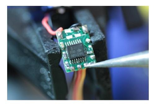
We're going to trick the servo driver into thinking that the potentiometer is always at a center-position with a pair of resistors.
