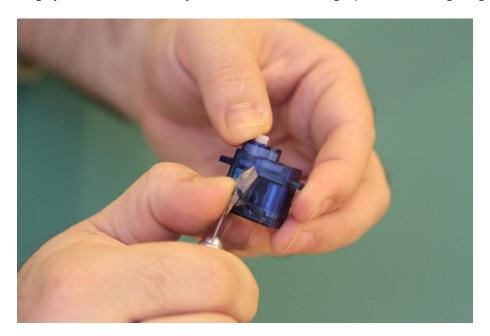
Remove any screws or bands that hold the servo case together.
