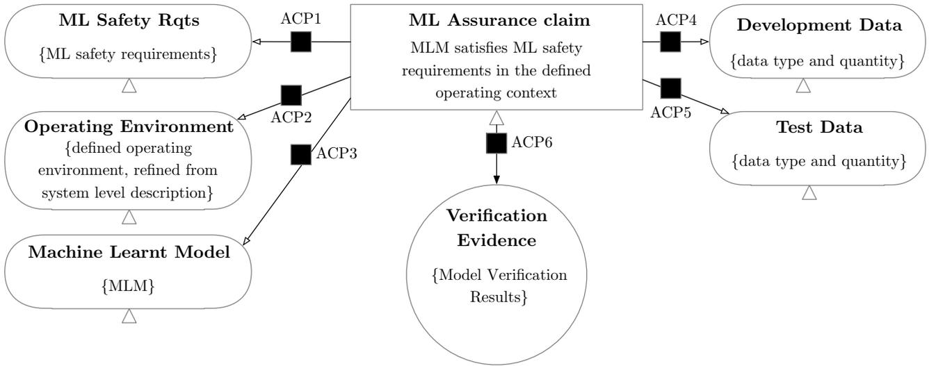
Figure 1: Safety Assurance Argument Pattern for a Machine Learned Model
