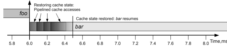
Fig. 7. If the addresses to be fetched are known in advance, and the memory subsystem is pipelined, the total time to restore the cache state of bar is 490\mu\text{s} , less than half the combined cost of individual cache misses in Figure 6.
