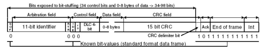
**Key point:** Message Identifier determines priority for access to bus (11-bit or 29-bit identifiers for messages which must be unique)
