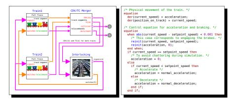
Fig. 6. FMI cosimulation (left) and train control equations (right).
