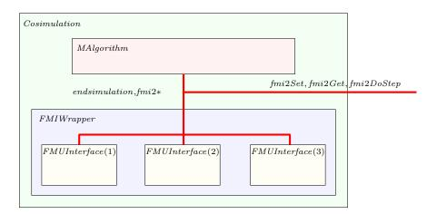
Fig. 2. Structure of a co-simulation model
