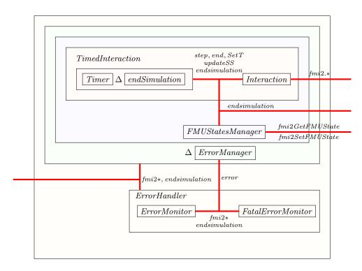
Fig. 3. Structure of a model of a master algorithm
