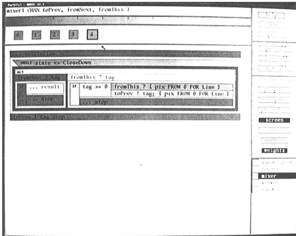
Now most of the work in the ALT is in the branch taking input from its own worker process. The only work done in the other branch is the receipt of the “stop” signal. There are no results (indicated by a white box), since there are no Transputers further down the pipe sending them on.
