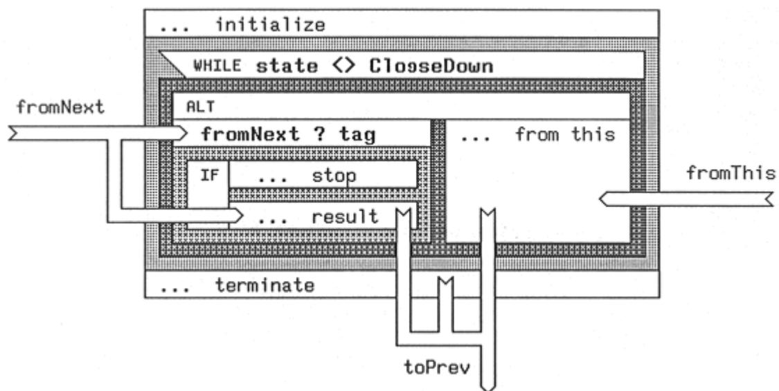
Here you can see the way GRAIL draws IFs and ALTs. Channels entering and leaving folds show up clearly.
