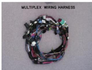
Prior to the 1990s, cars used point-to-point wiring. This was expensive to manufacture, install and maintain. From 1991, the automotive industry began to use Controller Area Network (CAN) [1] to connect Electronic Control Units (ECUs) such as engine management and transmission control. Using this approach dramatically reduced the size, weight and complexity of the wiring harness, for example with CAN, a door system in a high-end car typically requires 4 wires, compared
