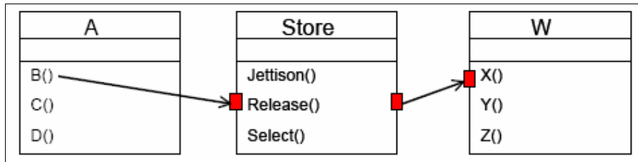
Figure 6 - Example of Class Diagram Showing Interactions and Constraints (Bates, Hawkins and McDermid 2003)
