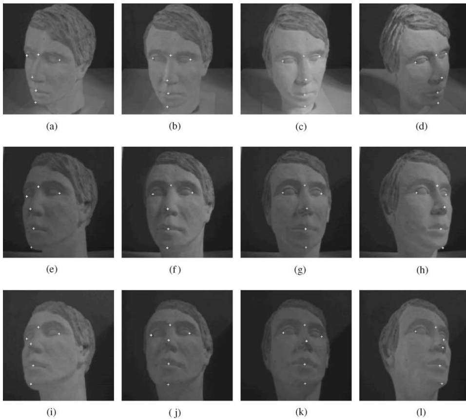
Fig. 15. A series of views of a plaster bust in which the camera direction is approximately fronto-parallel, oblique from above and oblique from below. The ground-truth angles are denoted by “T” and the estimated angles by “E”. (a) T: -30 E: -29.2 . (b) T: -10 E: -9.8 . (c) T: +10 E: +14.8 . (d) T: +30 E: +31.7 . (e) T: -30 E: -32.7 . (f) T: -10 E: -9.6 . (g) T: +10 E: +12.3 . (h) T: +30 E: +34.4 . (i) T: -30 E: -34.4 . (j) T: -10 E: -11.2 . (k) T: +10 E: +12.9 . (l) T: +30 E: +35.4 .
