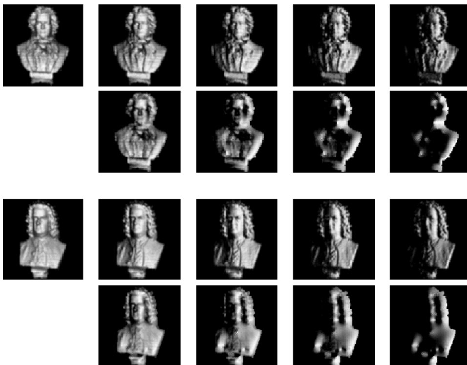
Fig. 2. Re-illumination results. The two sequences of images compare the results of re-illuminating the two busts using the surface normals extracted directly from the range image and those extracted using shape-from-shading. In each sequence the single leftmost image is the frontal image of the bust, illuminated by a light source in direction \mathbf{s} = (0, 0, 1)^T . This image is used as input to our shape-from-shading scheme. The recovered needle-map is then re-illuminated. In each sequence the top row shows the illumination of the range image for light-source directions of (left-to-right) 0^\circ, 20^\circ, 40^\circ, 60^\circ, 80^\circ to vertical in the x direction. The lower row shows the corresponding re-illumination results obtained using shape-from-shading.
